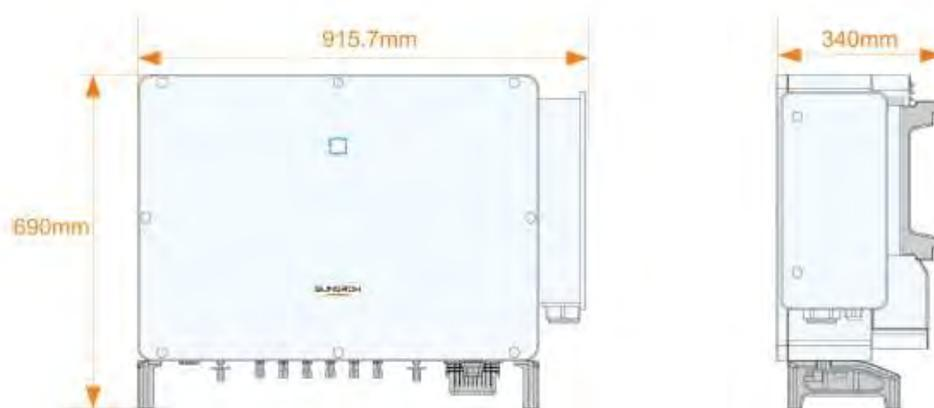
Figure 2-3 Dimensions of the Inverter (in mm)
