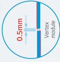
High density encapsulation technology, optimizing power output with good balance between reliability and efficiency, module efficiency increase **0.2~0.3%**
