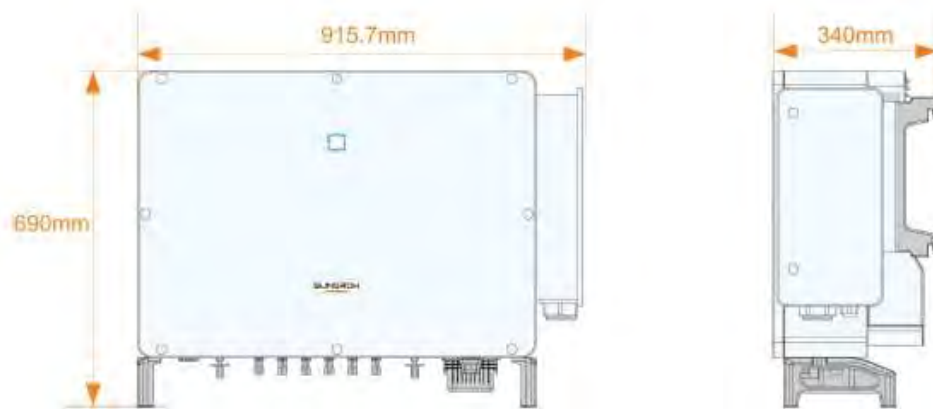
Figure 2-3 Dimensions of the Inverter (in mm)
